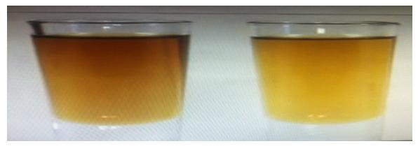
The old formula motor oil seen on the left, had many impurities. Our engines have tolerances to allow for the impurities which are no longer present. Today's oil seen on the right are very clean allowing for play in your engine.
